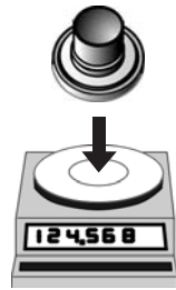
Figure 5. Weigh cassette with filter on a five-figure balance.
