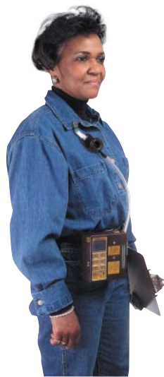
Figure 12. IOM Sampler and pump on worker
