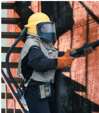
Worker Wearing Abrasive Blasting Sampler for Heavy Metals
