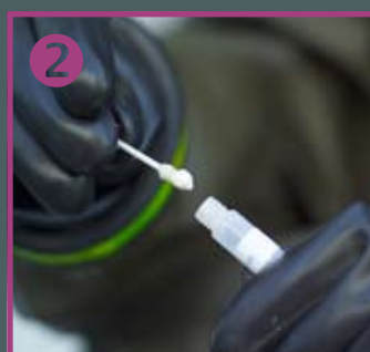
2 Extract the sample in buffer solution.
