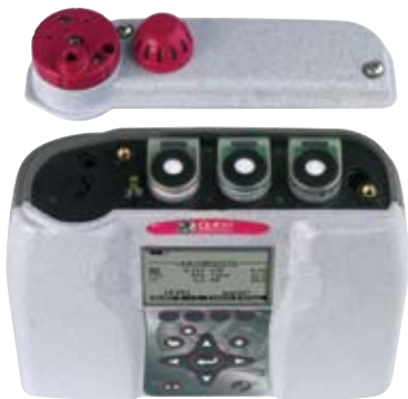
Removable sensor bar for easy access to sensors
