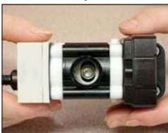
Correct: Eccentric centered in yoke.
