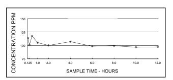
Concentration values are calculated using the 1 through 8 hour time-weighted average sampling rate of 13.7 ml/min based on a standard atmosphere of 98.7 ppm (calculated, checked by two reference methods).
