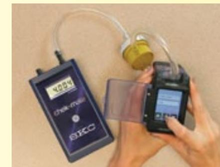
1 **Set and verify** pump flow rate using the kit calibrator.
