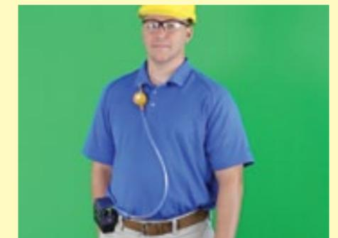
3 **Collect a sample** by running the pump for the work shift or other desired sampling period.
