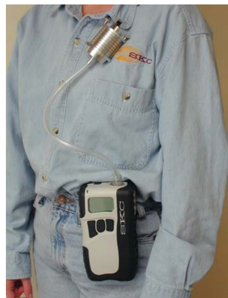
Sioutas Personal Cascade Impactor in Sampling Train
