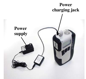
Leland Legacy charging train
