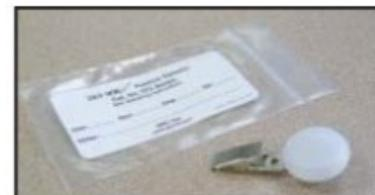
Write the date, start time, and sampler ID number (found on the sampler) on the label on the pouch.
