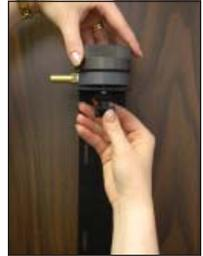
3. Insert screw on rain cover into screw hole in top of impactor inlet and rotate cover until tight.
