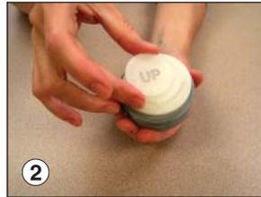
Place impaction disc on filter cassette top. The rough side of the impaction disc should face up. SKC-supplied discs are stamped with "UP" on the appropriate side.
