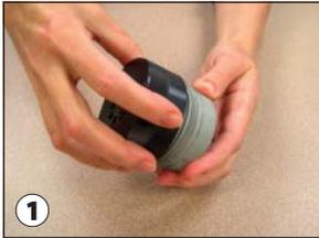
Unscrew impactor inlet from exhaust.
