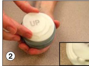
Locate recessed area on filter cassette top and remove impaction disc. If chemical analysis of larger particles is desired, place in appropriate container for shipping to a laboratory for analysis. See *Ordering Information, Accessories for Glass Jars*.
