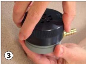
Place filter cassette on exhaust and screw impactor inlet and exhaust together just until tight. Further hand-tighten by 1/4 turn only.
