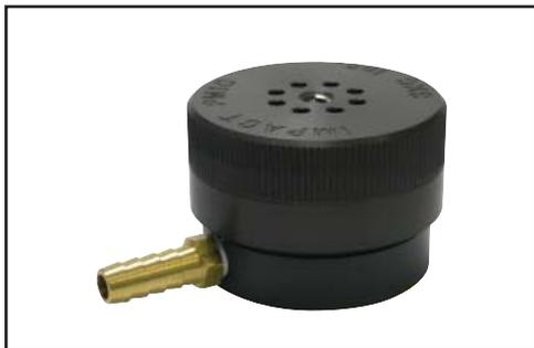
The patented\* IMPACT Sampler is an inertial impactor designed to remove particles larger than its cut-point by capturing them on a disposable oiled impaction disc that reduces particle bounce. Particles that are smaller than the cut-point are collected on a 47-mm filter. The IMPACT Sampler mounts easily and makes media changes fast and simple with its convenient removable filter cassette.
