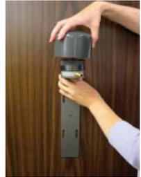
5. After the desired sample time has elapsed, turn off the pump and record sample stop time and other pertinent data.
