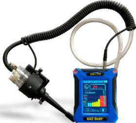
SM-7204 is uniquely optimized for silica exposure measurement at the new PEL.
