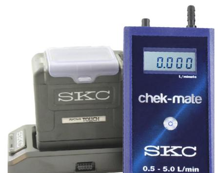
Automatic flow rate verification/calibration with CalChek
