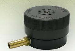
The patented\* SKC IMPACT single-stage inertial impactor is designed for efficient collection of PM10, PM2.5, or PM Coarse (10-2.5) in ambient air. Operated at 10 L/min constant flow, larger particles are captured on a disposable pre-oiled impaction disc while smaller particles collect on a 47-mm filter. The filter and impaction disc are housed in a removable filter cassette. The IMPACT's higher flow rate provides increased sensitivity for low levels of PM.
