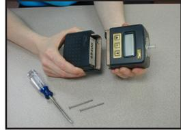
2. Insert and tighten two security screws provided.
