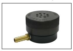
The patented\* IMPACT Sampler is an inertial impactor designed to remove particles larger than its cut-point by capturing them on a disposable oiled impaction disc that reduces particle bounce. Particles that are smaller than the cut-point are collected on a 47-mm filter. The IMPACT Sampler mounts easily and makes media changes fast and simple with its convenient removable filter cassette.
