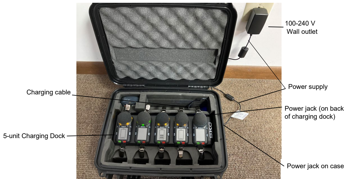
Figure 2b. Charging Train in Carry Case with Charging Cable Installed
