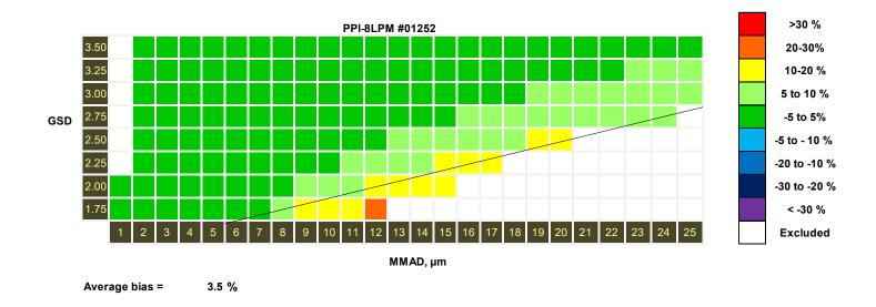
Figure 2c. Bias map for the SKC 8-L/min-PPI impactor (#01252) for different particle size distributions (MMAD and GSD).
