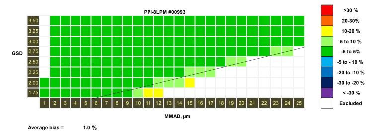
Figure 1c. Bias map for the SKC 8-L/min-PPI impactor (#00993) for different particle size distributions (MMAD and GSD).
