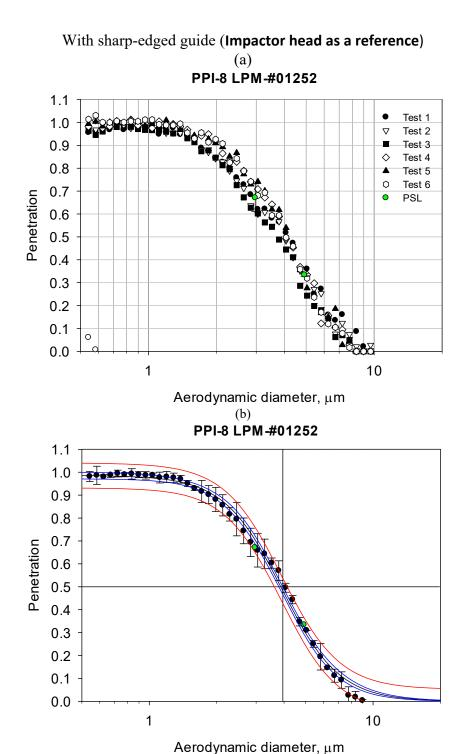
Figure 2. SKC PPI-8 L/min impactor penetration curve as a function of particle size: a) individual data points of the six tests and b) average values and standard deviations for each particle size based on six tests.
