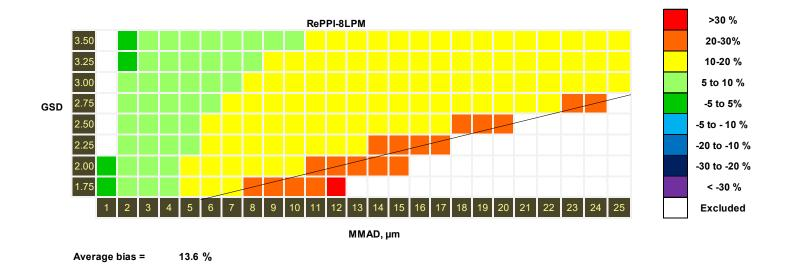
Figure 3c. Bias map for the SKC 8-L/min-RePPI Impactor for different particle size distributions (MMAD and GSD).
