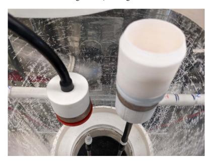
Picture 3. Location and orientation of PPI-8 L/min impactor in the test chamber when it was tested facing down. This test was performed with NaCl particles only.
