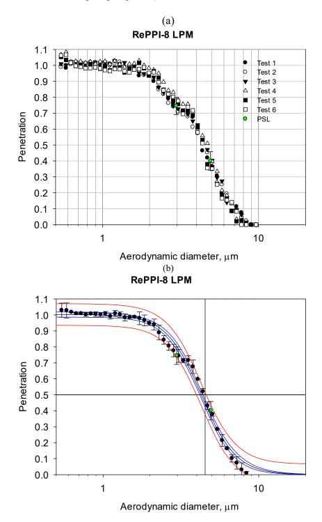
Figure 3. SKC RePPI-8 L/min impactor penetration curve as a function of particle size: a) individual data points of the six tests and b) average values and standard deviations for each particle size based on six tests.
