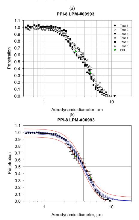
Figure 1. SKC PPI-8 L/min impactor's penetration curve as a function of particle size: a) individual data points of the six tests and b) average values and standard deviations for each particle size based on six tests.
