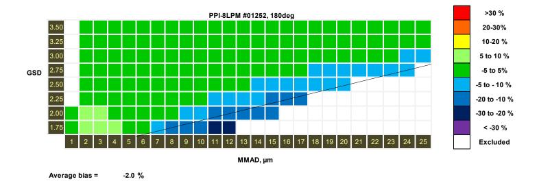
Figure 4c. Bias map for the SKC 8-L/min-PPI impactor (#01252) for different particle size distributions (MMAD and GSD) with the sampler facing down (180 degrees to the airflow).
