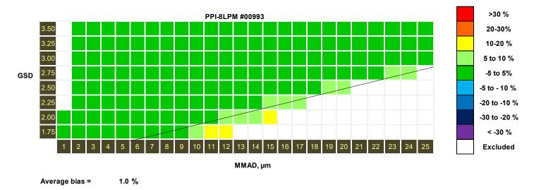
Figure 1c. Bias map for the SKC 8-L/min-PPI impactor (#00993) for different particle size distributions (MMAD and GSD).
