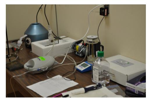
Figure : Sampling set up used in conducting experimental research. Displayed is the SKC BioSampler®, nebulizing unit, sampling pump, calibration equipment, reagents and centrifuge.
