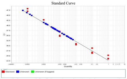
Figure : ABI StepOne<sup>TM</sup> standard curve graph for all air sample reactions. Standard curves are used to determine the absolute quantity of *B. abortus* in an air sample. Each red bar represents a known standard dilution concentration (1:10 dilution), while each blue bar represents an unknown experimental air sample concentration. Curves are generated by plotting fluoresce threshold cycle (y-axis) to quantified concentrations (x-axis).
